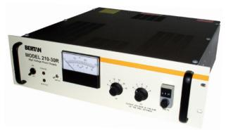
Spellman's Bertan brand of 210 Series of 125 to 225 watt high voltage power supplies provide regulated high voltage outputs from 1 to 50kV. The low noise, linear topology employed results in extremely low output ripple specifications. Units are inherently reversible by design, providing either positive or negative output polarity. The 210 is fully arc and short circuit protected. Excellent regulation specifications are featured along with outstanding stability performance.
